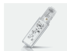
Bluetooth Connector for remote desk control
